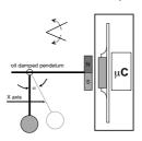
Pendulum damping: by oil filling
